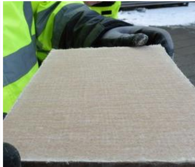
Figure 2: Photo of 8 mm thick MgO-board with a glass fibre mesh on both surfaces.
